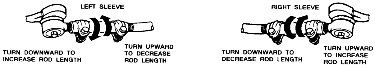
Figure 12-20.—Adjustments for toe-in and steering wheel alignment.
